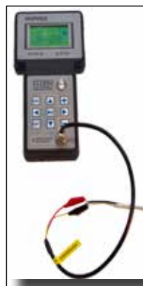
ETT985 Connected to transducer
